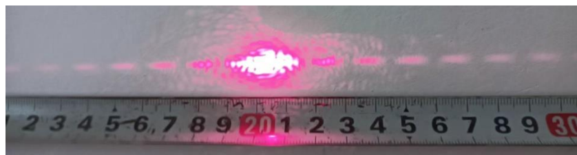
Figure 8. Fringe images with baffle - filament distance from 5 mm to 0.3 mm
