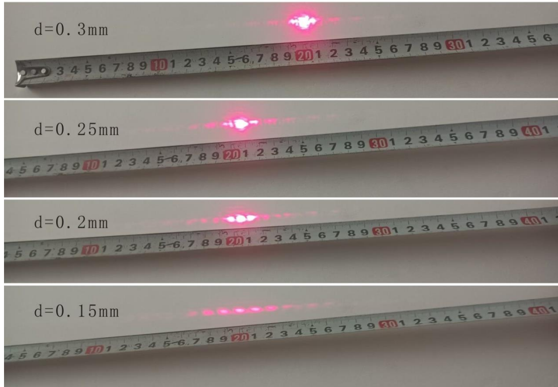
Figure 5. Sequence of fringe changes under symmetrically reduced slit width
