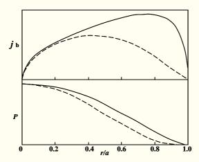
**Fig. 2** Typical bootstrap currents with a shift due to r/a where r is the radial direction of the Tokamak, and a is the inner radius of the Toroid This figure is reproduced from Wesson [29] Then one has
