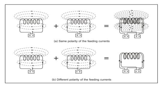
Figure 1. Two-solenoid experiment.
