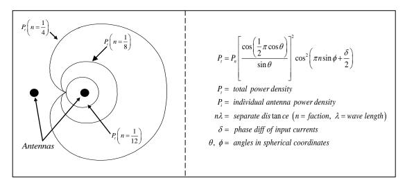
Figure 3. Radio radiation patterns of a two half-wave antennas & the formula.
