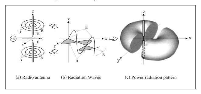
Figure 8. Electromagnetic waves radiation process.
