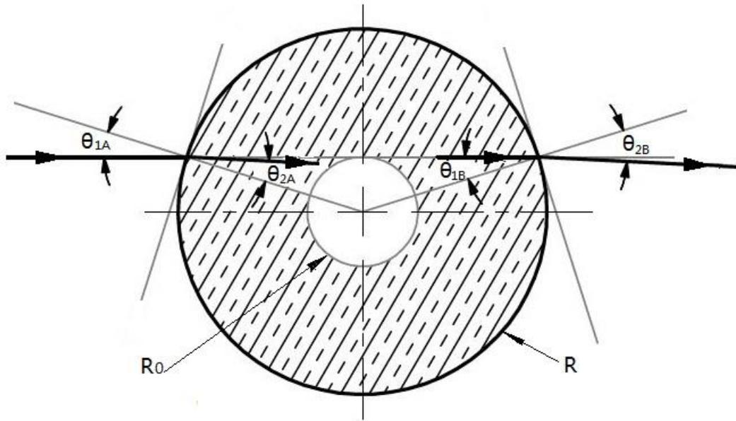
Figure 4.3 Deflection angle of light under sun's atmosphere
