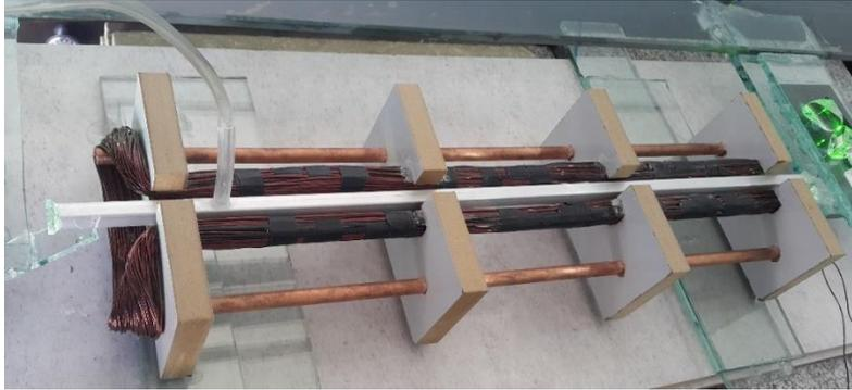
**Fig. 8.** Longitudinal electrical magnet with two parallel rows of a coiled wire
