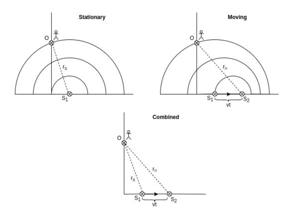
Figure 3: Doppler shift for a moving source
