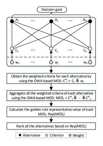
Fig. 5. Hierarchical structure of the proposed decision method based on the developed MOC algorithm.
