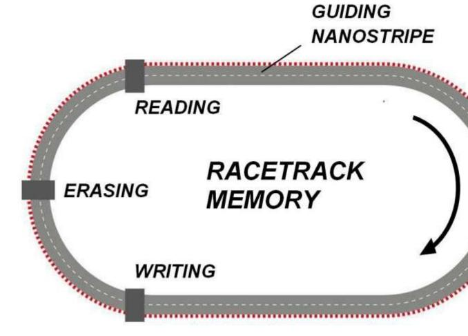
The concept of racetrack memory: magnetic objects move from writing to reading elements. Credit: Forschungszentrum Jülich
