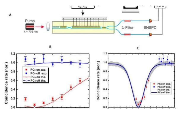
Experimental setup and quantum results. (A) Experimental setup for quantum characterization of the active HOM chip. A tunable narrowband continuous-wave pump laser around 776 nm is coupled into the channel with the PDC source. To avoid ...<u>more</u>
