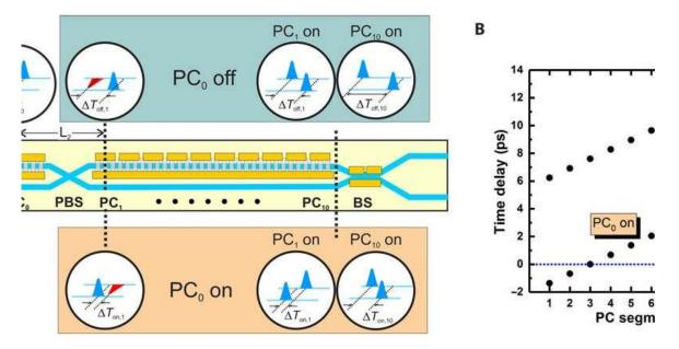
Illustration of the principle of the adjustable BED line. (A) The diagram shows the chip design together with some insets illustrating the temporal relation of the horizontally (red) and vertically (blue) polarized photon wave packets at ...<u>more</u>
