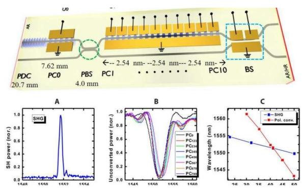
Upper panel: Schematic illustration of the integrated quantum optic chip with monolithic inclusions of a PDC source (20.7 mm), electro-optic PCs (7.62 mm), PBS, highlighted in green (4.0 mm), BS highlighted in blue, and a single element of ...<u>more</u>
