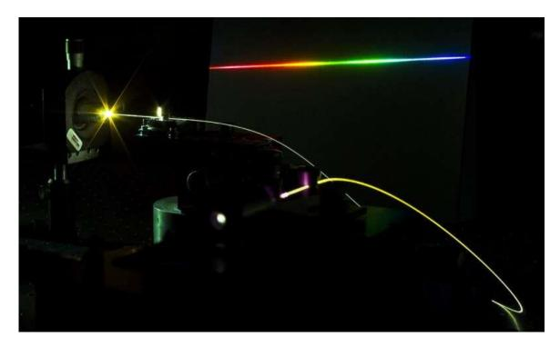
An ultrashort pulse is sent into an optical fibre and produces new frequency components via intense light-matter interactions. The progressive spectral broadening of the initial light pulse occurring during propagation, ultimately leads to ...more
