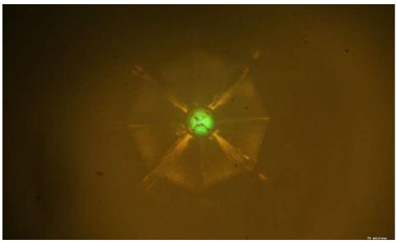
Scientists bombarded a sample of a new superconducting material with X-rays to study its structure at the Advanced Photon Source at Argonne National Laboratory. The X-ray fluorescence creates the greenish color at the sample (center). Credit: Drozdov et al.
