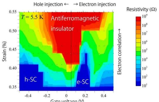
Resistivity is shown by colors. The insulator region (red) is surrounded by the superconducting regions (blue). The shapes of the insulating and superconducting regions differ between the negative and positive ranges of the gate voltage. The shape of the electron-doped superconducting region (e-SC) is found to be quite anomalous. Credit: NINS/IMS
