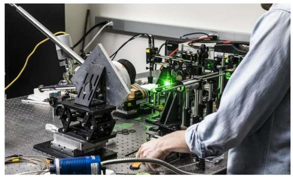
University of Washington postdoctoral researcher Matthew Crane operates equipment that uses a laser to heat the gasket of a high-pressure diamond anvil cell above 3,100 F, more than one-third the temperature of the sun. Credit: Mark Stone/University of Washington
