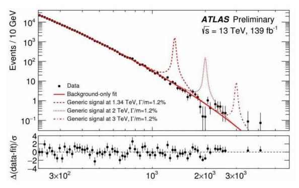
Measured dielectron mass distribution for the data (black points), together with the total background fit result is shown (red continuous line), with various possible Z' signal distributions overlaid (dashed red line). The sub-panel shows ...more
