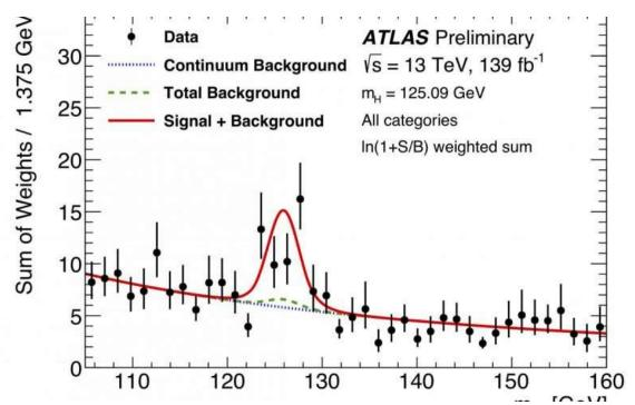
The ttH signal in the diphoton invariant mass spectrum. Events from the different analysis categories are weighted according to the category sensitivity to the ttH signal. The ttH signal manifests itself as a localised resonant bump in the red curve, representing the fit to the data of the signal and background shapes. The other Higgs production modes provide a small contribution to the resonant peak, as shown by by the green dashed line. Credit: ATLAS Collaboration/CERN
