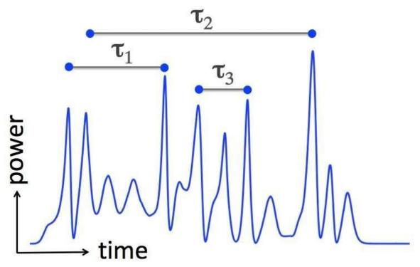
Simulated profile of an X-ray pulse from an X-ray free-electron laser. It consists of a train of narrow spikes whose intensity (power) fluctuates randomly. SLAC researchers suggest using pairs of these spikes for pump-probe experiments that trigger and measure structural changes in a sample, turning a former nuisance into an advantage. This example highlights three pairs of spikes with different time delays between them. Credit: SLAC National Accelerator Laboratory
