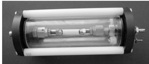
Fig 7. Vacuum cell with two glow discharge electrodes
