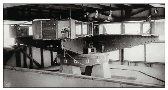
Figure 4. **Dayton Miller's light-beam interferometer**, at 4.3 meters across, was the largest and most sensitive of this type of apparatus ever constructed, with a mirror-reflected round-trip light-beam path of 64 meters. It was used in a definitive set of ether-drift experiments on Mt. Wilson, 1925-1926. Protective insulation is removed in this photograph, and windows were present all around the shelter at the level of the interferometer light-path. [8]
