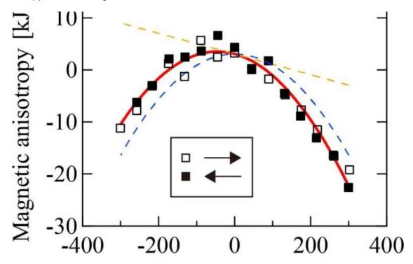
DC voltage dependence of the anisotropy of the magnetic pole of the free layer. The filled and open squares represent the voltage sweep direction. The red line is the fitting of the data. The yellow and blue dashed lines represent the ...more
