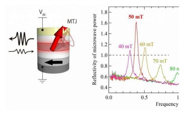
Schematic of the microwave amplification (left) and magnetic field dependence of the microwave power reflectivity spectra (right). The reflected microwave is amplified by the dc voltage (Vdc) biased MTJ. In our experiment, we have obtained ...more
