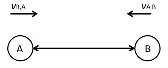
Fig.1 Two inertial observers A and B in relative motion. The velocity  $v_{B,A}$  is that of observer B as measured by observer A,  $v_{A,B}$  is that of observer A as measured by observer B.
