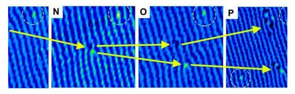
Cooling sample. The yellow arrows indicate the vortex-antivortex pair, as it is generated (N), separates (O), and further diverges (P). The authors note that the process is observed at domain junctions called Y dislocations (as in M) or on ...<u>more</u>
