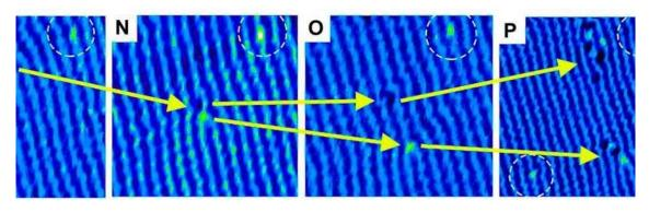
Cooling sample. The yellow arrows indicate the vortex-antivortex pair, as it is generated (N), separates (O), and further diverges (P). The authors note that the process is observed at domain junctions called Y dislocations (as in M) or on ...<u>more</u>
