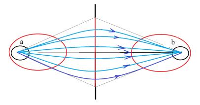
Figure 23: The mutual energy flow between the two point  $\boldsymbol{a}$  and  $\boldsymbol{b}$ . Assume there is a partition board. This wave is quasi-plane wave.
