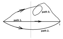
Figure 20: In the figure there are 3 paths. Path (1) is straight line. The path (2) is a streamline, this is a line the mutual energy flow will go. The path (3) path is arbitrary path.
