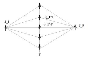
Figure 14: Huygens virtual source, which can replace the field, i.e.,  $\xi_I^{\Gamma} \Longleftrightarrow \sigma_I^{\Gamma}$
