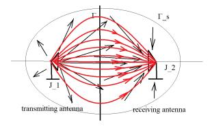
Figure 13:  $J_1$  is inside  $V_1$  which is a transmitting antenna and sends the retarded wave out.  $J_2$  is inside  $V_2$ , which is a receiving antenna and sends advanced wave out. The mutual energy current go to outside of the surface  $\Gamma_s$  is 0. The mutual energy current go through  $\Gamma$  is a constant,  $\Gamma$  can be in any place between  $V_1$  and  $V_2$ . The red arrowhead is the mutual energy flow which is sent out from  $V_1$  and has been received in  $V_2$
