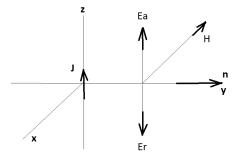
Figure 15: The fields produced by a current source. The magnetic field produced by the current can be decided by the right hand law, and hence only in one direction showed as  $\boldsymbol{H}$ . There two possibility, for the electric field. It can direct up or direct to down. The the up direction electric field is the retarded field  $\boldsymbol{E}_r$  and the down direction electric field is the advanced field  $\boldsymbol{E}_a$ .
