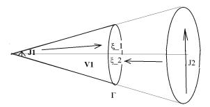
Figure 19: The wave inside cone beam wave guide. Assume there is a source  $J_1$  which sends the retarded filed  $\xi_1$  and a load  $J_2$  which sends the advanced wave  $\xi_2$ . In this wave guide, we can calculate the energy flow with Maxwell equations and Poynting theorem or calculate the energy flow with mutual energy flow.
