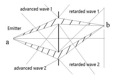
Figure 24: Assume there is a partition board which is put between the point a and b. Double slits are opened on the partition board which allow the particle to go through. The shape of the mutual energy flow for the double slits are shown.
