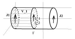
Figure 18: The wave inside the wave guide. Assume there is a source  $J_1$  which sends the retarded filed  $\xi_1$  and a load  $J_2$  which sends the advanced wave  $\xi_2$ . In this wave guide, we can calculate the energy flow with Maxwell equations and Poynting theorem or calculate the energy flow with mutual energy principle.
