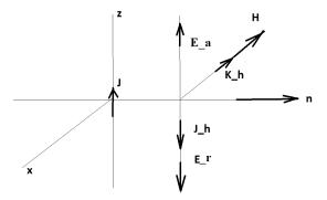
Figure 16: The fields produced by a current source. In the place close to the current source, there are a infinite plane  $\Gamma$ . The field produced by the source  $J_I$  can be described by  $\xi_I^{\Gamma}$ . This field can also be described as Huygens virtual sources  $\sigma_I^{\Gamma} = [J_I^{\Gamma}, K_I^{\Gamma}]$ .
