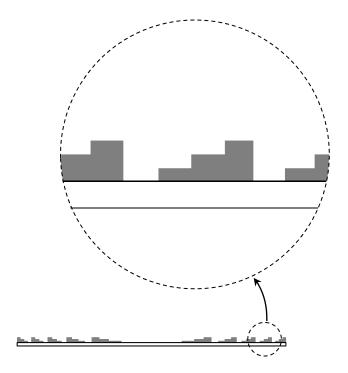
Figure 3. Cross-section of a stepped, 4-level phase-Fresnel lens.
