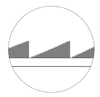
Figure 7. Single-sided EUV lens with 15 layers.
