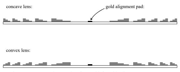
Figure 9. concave and convex lens forms with frontside alignment targets
