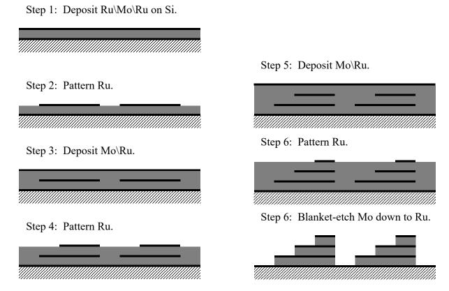
Figure 8. e-beam patterning steps for lens manufacture
