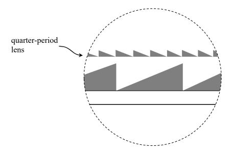
Figure 4. Two stacked phase-Fresnel lenses, equivalent to the stepped-profile lens of Fig. 3.
