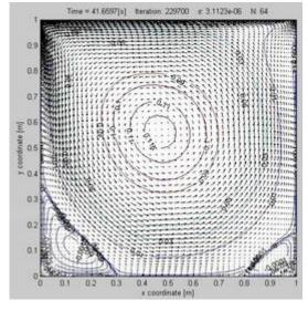
In the 2 last images, are the representations of pressure lines in a cavity with a fluid in movement.
