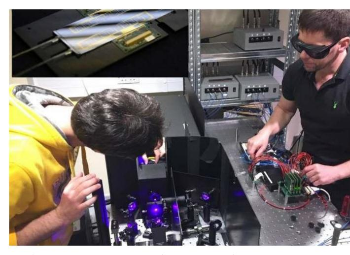
Dr Laing's laboratory where the experiments were performed. Single photons of light are generated using a powerful Ti-Sapphire laser, to pump a series of nonlinear crystals, operated by Ph.D. student and co-author Nicola Maraviglia (left). ...more
