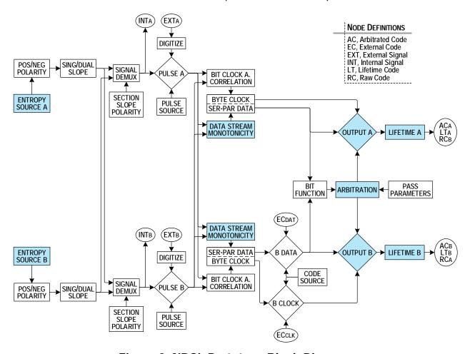
Figure 2. NRCL Prototype Block Diagram
