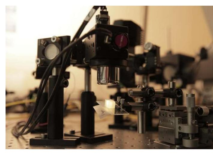
This custom-built optical coherence tomography instrument uses visible light to view tissue. Credit: Renee Meiller
