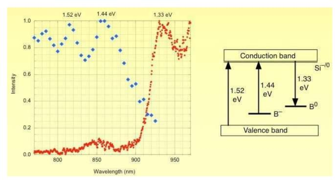
Left: Excitation curve (blue diamonds) and emission curve (red circles) showing that almost all of the emission spectrum of the GaAs scintillator is outside the absorption band. Right: Simplified diagram of excitation and emission ...more
