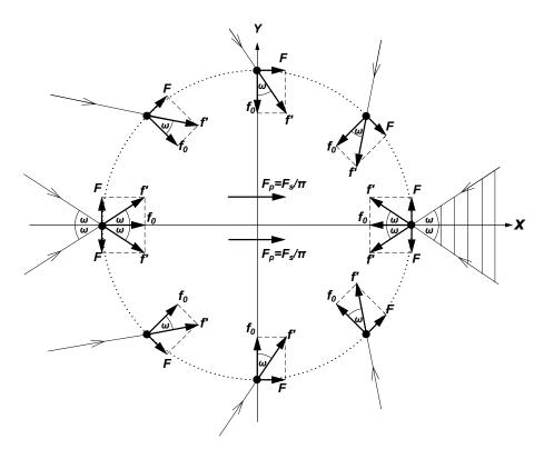
**Figure 1.** Accumulation of motion force F on the particle spherical zone
