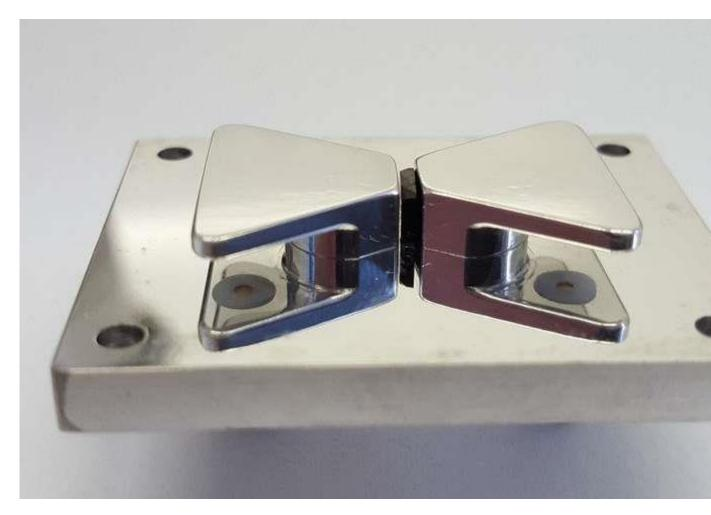
The microwave resonator with the diamond in the middle. Because of the lattice defects, the diamond is black. Credit: Vienna University of Technology
