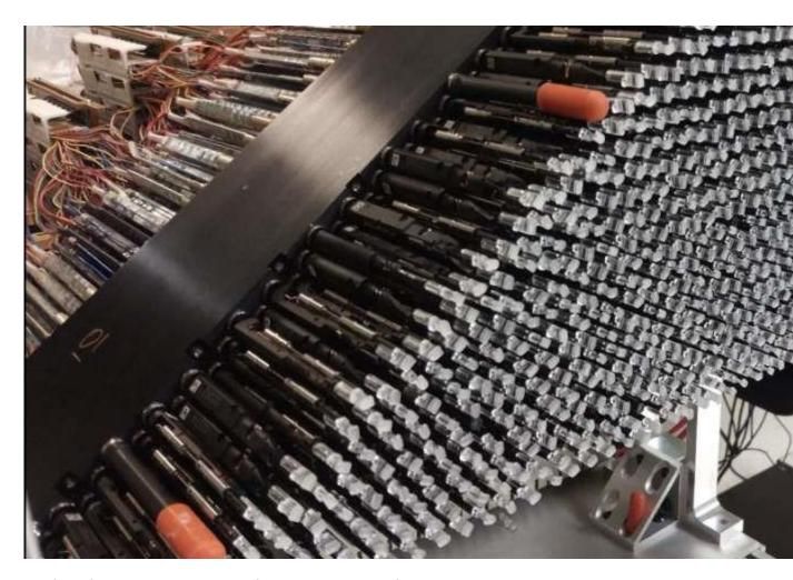
The first of 10 wedge-shaped petals for the DESI project is fully stocked with 500 slender robotic positioners. These positioners will each swivel independently to gather light from a preprogrammed sequence of space objects, including ...more
