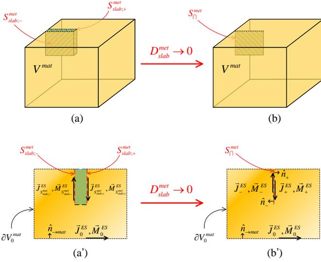
Fig. 3. (a) A thick metallic slab is submerged into material body; (b) a metallic surface is submerged into material body; (a') the sectional view of Fig. 3 (a), and the equivalent surface currents  $\{\vec{J}_{slab,+}^{ES}, \vec{M}_{slab,+}^{ES}\}$  and  $\{\vec{J}_{slab,-}^{ES}, \vec{M}_{slab,-}^{ES}\}$ ; (b') the sectional view of Fig. 3 (b), and the equivalent surface currents  $\{\vec{J}_{\pm}^{ES}, \vec{M}_{\pm}^{ES}\}$  and  $\{\vec{J}_{\pm}^{ES}, \vec{M}_{\pm}^{ES}\}$ .
