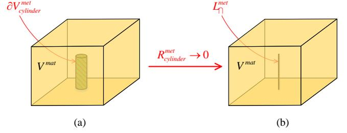
Fig. 4. (a) A metallic cylinder is submerged into material body; (b) a metallic line is submerged into material body.
