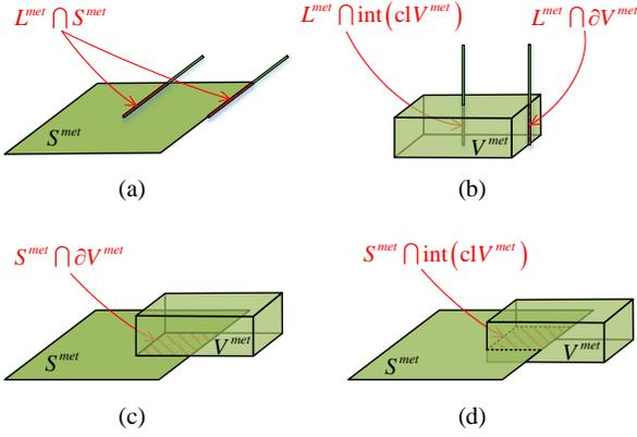
Fig. 2. (a) A part of metallic line contacts with metallic surface, and this case is not considered in this paper; (b) a part of metallic line contacts with or is submerged into metallic body, and this case is not considered in this paper; (c) a part of metallic surface contacts with metallic body, and this case is not considered in this paper; (d) a part of metallic surface is submerged into metallic body, and this case is not considered in this paper.
