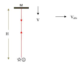
Assume that the mirror is moving towards or away from the source and the observer with velocity V, with the source and observer at rest relative to each other, but with a common absolute velocity as shown in the next figure. The absolute velocity vector can have any magnitude and direction. How are such experiments analyzed?
