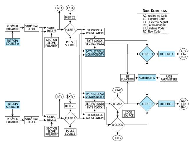
Figure 2. NRCL Block Diagram
