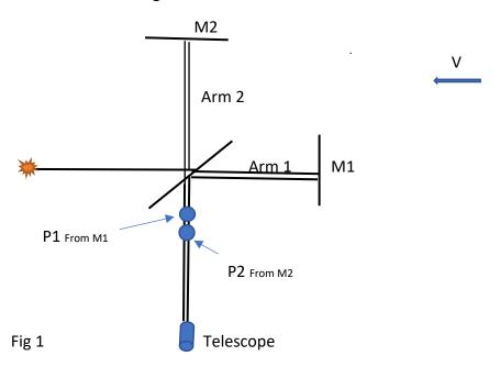
When the interferometer is turned through 90°, the corpuscle that travels through arm 1, which is now perpendicular to the direction of the motion of the earth, arrives earlier than the one going through arm 2. (calculations show that it takes longer for the light to travel through the arm parallel to the direction of the motion of the earth than the light going through the perpendicular direction). See Fig 2.
