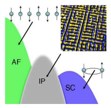
An "antiferromagnetic" state, where the magnetic moments of electrons are opposed, can lead to a variety of unexpected arrangements of electrons in a high-temperature superconductor, then finally to the formation of "Cooper pairs" that conduct without resistance, according to a new theory. [22]
