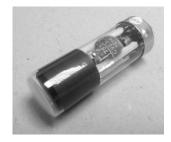
FIG. 1. A CV2302 28 mm cathode ray tube. Photo credit: langrex.co.uk.
