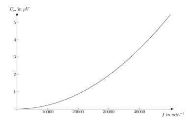
Figure 3: Expected voltage  $U_m$  for  $R_i = 10cm$ ,  $R_o = R_i + 3mm$ ,  $R_g = 30cm$ , d = 3mm and  $U_c = 10kV$  in dependency of the rotational speed  $f = \frac{\omega}{2\pi}$ .
