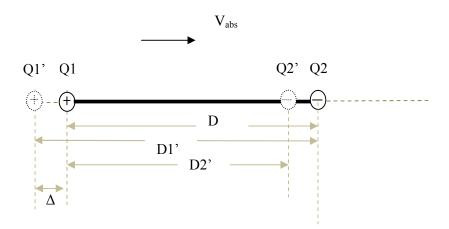
D is the actual, physical distance between real charges Q1 and Q2. D1' is the apparent distance of Q1 as seen by Q2. We can also say that D1' is the distance of apparent charge Q1' from real charge Q2. D2' is the apparent distance of Q2 as seen by Q1. We can also say that D2' is the distance of apparent charge Q2' from real charge Q1.
