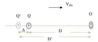
Although the charge is physically at Q, it appears to the observer that the charge is at Q'. There will be an apparent change of charge position as seen by the observer. The charge appears to have shifted backwards, away from the observer.
