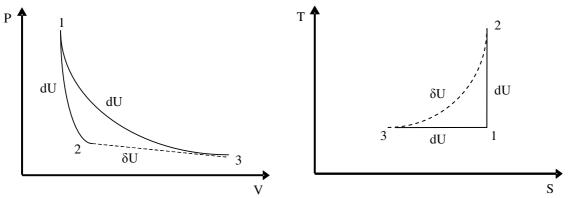
Figure 5 – Illustrative P-V and T-S diagrams for an one reservoir engine
