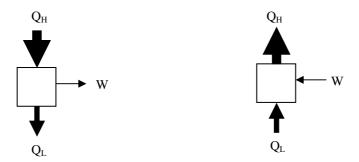
Figure 1 – Carnot heat engine and refrigerator
