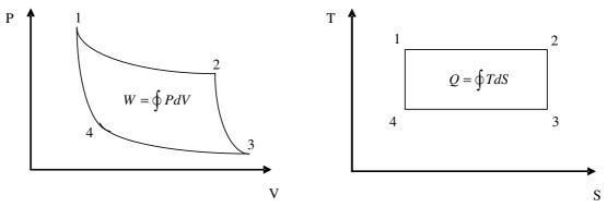
Figure 2 – P-V and T-S diagram of Carnot heat engine or refrigerator
