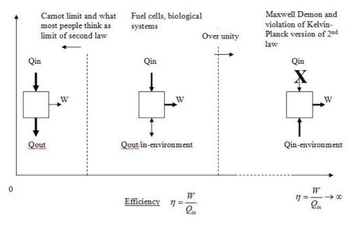
Figure 3 – The continuum of heat engines
