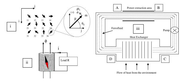
Figure 7i,ii,iii – The basic flux collapse power generation method and plant diagram
