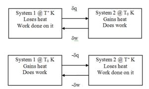
Figure 4 – Statistical fluctuation in temperature with micro-heat and micro-work flows
