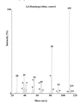
Figure 4. GC-MS spectrum of control sample of 2,6-diaminopyridine.
