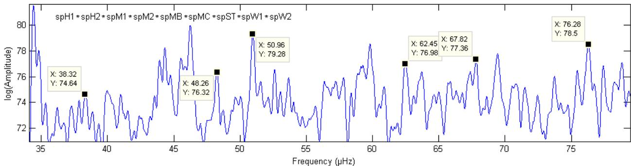
At least six prominent peaks in the frequency range of interest can not be assigned to known causes<sup>[3]</sup> and were investigated in detail. But the identification of unusual frequencies with striking good SNR is not sufficient, there are additional constraints to convince with the result.
