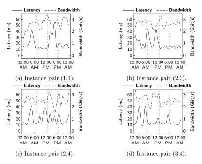
Figure 1: Network interconnection speed (latency and bandwidth) between four pairs of cloud instances. The three dotted vertical lines indicate the approximate times at which the interconnection matrices shown in Figure 2 were generated.
