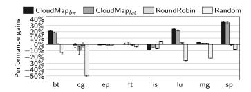
Figure 6: Performance gains on 8 A7 instances (64 tasks), normalized to the default mapping policy, with input size B.
