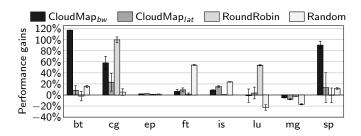
Figure 9: Performance gains on 32 A7 instances (256 tasks), normalized to the default mapping policy, with input size C.
