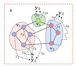
Diffusion estimation in a sensor network. In this graphical examples, the network is composed by 8 nodes, dividing in 3 clusters and providing 3 different vectors of measurements  $y_1$ ,  $y_2$  and  $y_3$ . In this case,  $\mathcal{Y} = \mathbf{y}_1 \cup \mathbf{y}_2 \cup \mathbf{y}_3$ ,  $\mathbf{y}_j \cap \mathbf{y}_k \neq 0$  for  $j \neq k$  (in this case,  $d_{Y_1} = 5$ ,  $d_{Y_2} = 3$ ,  $d_{Y_3} = 2$ ). Each sensor can provide more than one measurement.
