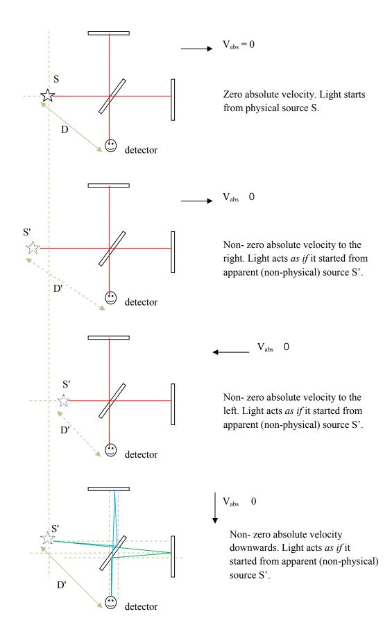
No (significant) fringe shift will be expected simply because the source position has changed.
