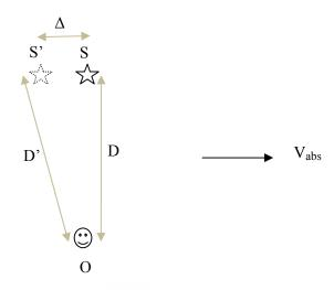
During the time interval that the light pulse goes from S' to O, the source goes from S' to S.
