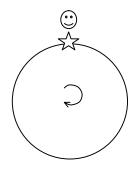
Assume that the light source emits light in the opposite directions tangentially. The two light beams travel in circular paths in opposite directions before being detected at the detector. A circular mirror is used to make light travel in circular path.
