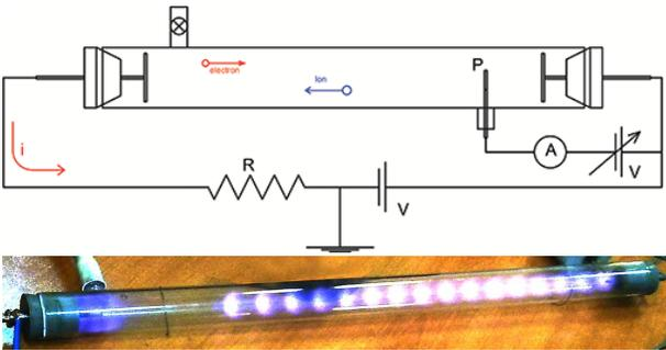
FIG. 2: The figure shows Langmuir Probes experiment, this experiment is used to obtain the properties of plasma including the speed of free electron.
