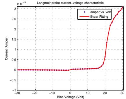
FIG. 3: The figure shows I-V properties of Langmuir Probes experiment
