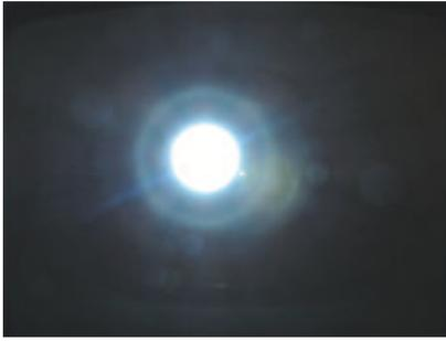
FIG. 5: It shows the image of electrons band in which halo effect is seen. This effect is only removed by fixed voltage and current.
