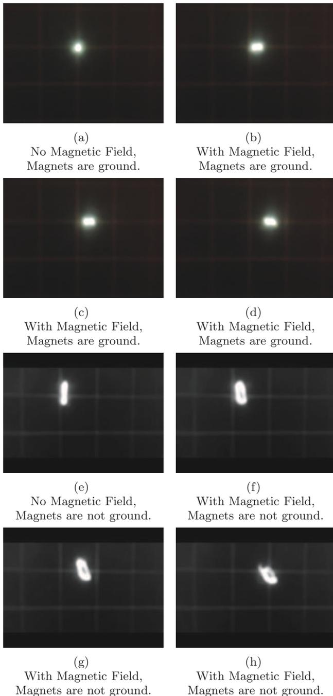
FIG. 7: The figure shows the move state of the electrons beam when electrons are affected by inhomogeneous magnet field both in adjoin of magnets to ground and non-adjoin them to ground.
