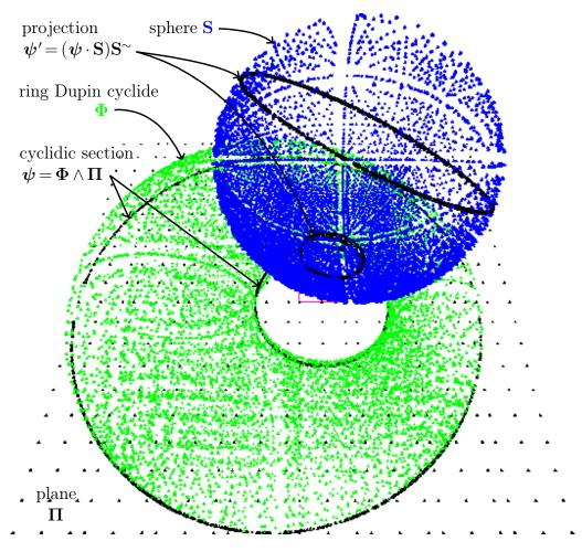
Figure 5. Projection of cyclidic section onto sphere
