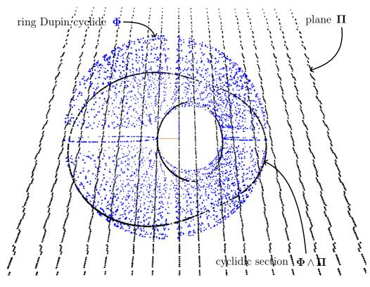
Figure 2. Cyclidic section: quartic plane curve
