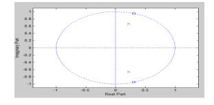
Figure 2 Poles and Zeros of the Notch Filter
