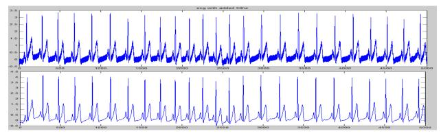
Figure 4 Application of Notch filter to ECG with PLI
