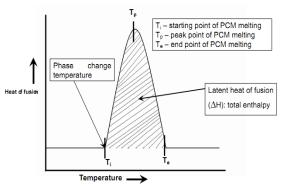
Fig. 3. Schematic of DSC heating thermogram of PCM. [21]
