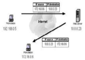
Figure 2: Spoofed source IP address
